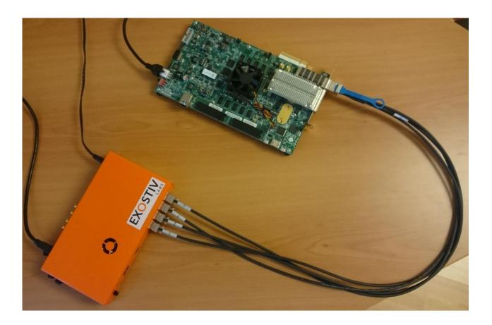
All the 4 transceivers of EXOSTIV Probe are connected with a 4xSFP+ to QSFP+ cable.
